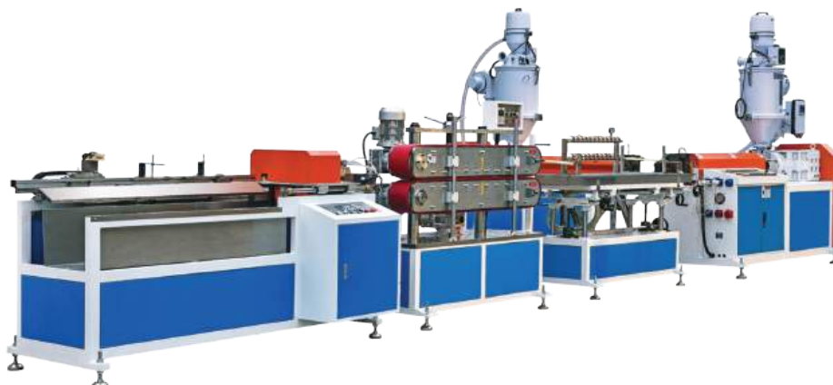
Diffuser Extrusion Machine
